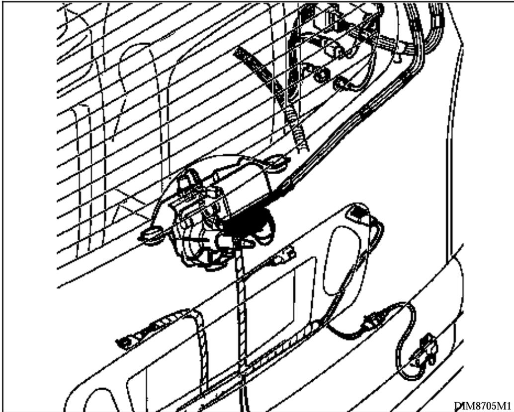
It receives the passenger compartment connection unit BII information concerning rear wiping, fog lights, closure of the tailgate and the rear screen position, rear passenger compartment and number plate lighting .
